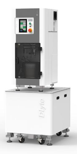
**D**Lyte11° series are the new patented machines for grinding and polishing Steel and Stainless-steel, Cobalt Chrome, Nickel, Titanium and Precious Metals.
