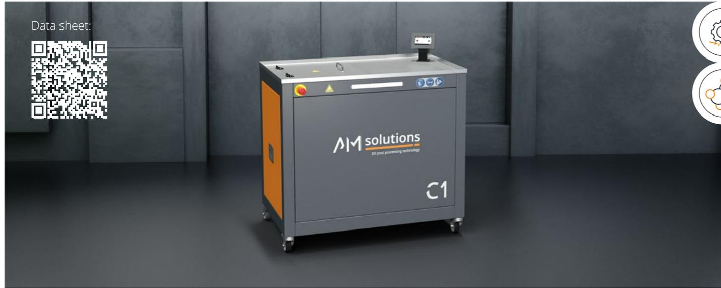
Our C1 system is an excellent tool for the automated and cost-efficient post processing of photopolymer components. The perfectly adapted compound and the interplay between mechanical and thermal effects results in a highly consistent, effective and gentle removal of support structures / resin. In addition, our C1 machine contains various features
